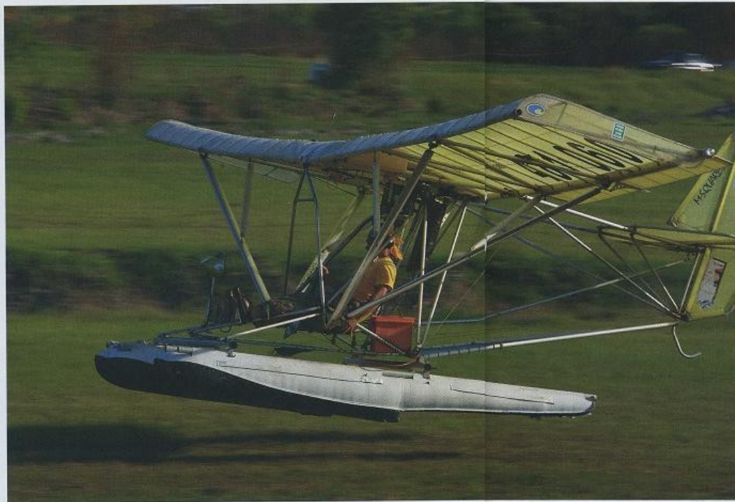
M-Squared specializes in float-equipped airplanes. This Breeze 2 SS (single-surface wing) is mounted on Full Lotus inflatable floats.
